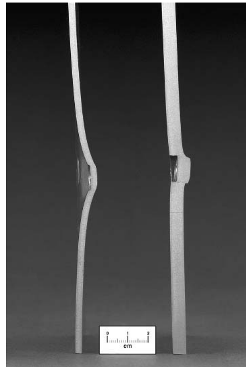
Fig. 6 Thin (3.2 mm) and thick (6.4 mm) 2024 Al panels tested just below the ballistic limit and sectioned through the center of the impact zone and viewed edge on. The thin panel (left) shows significant global plastic deformation of the panel. The thick panel (right) shows little global deformation with deformation and fracture dominated by shear plugging.
